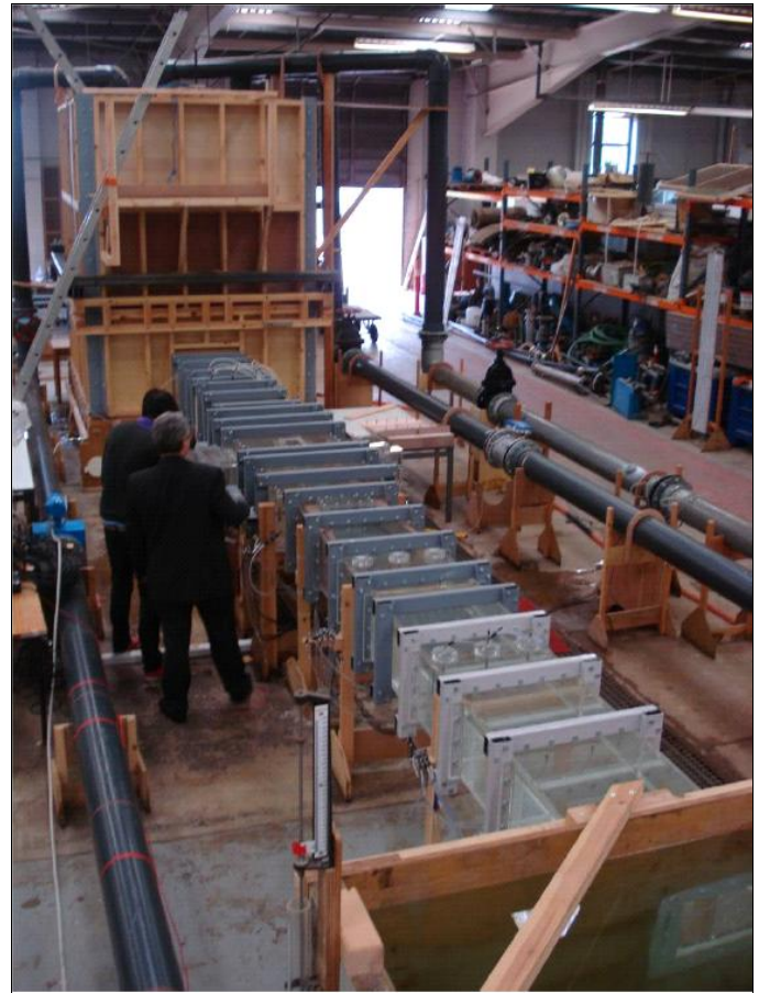
Figure 2: The VETT model at BHRGroup, showing a 3m header tank in the background; sink tank in the foreground and in between the acrylic model with steel bracing.
