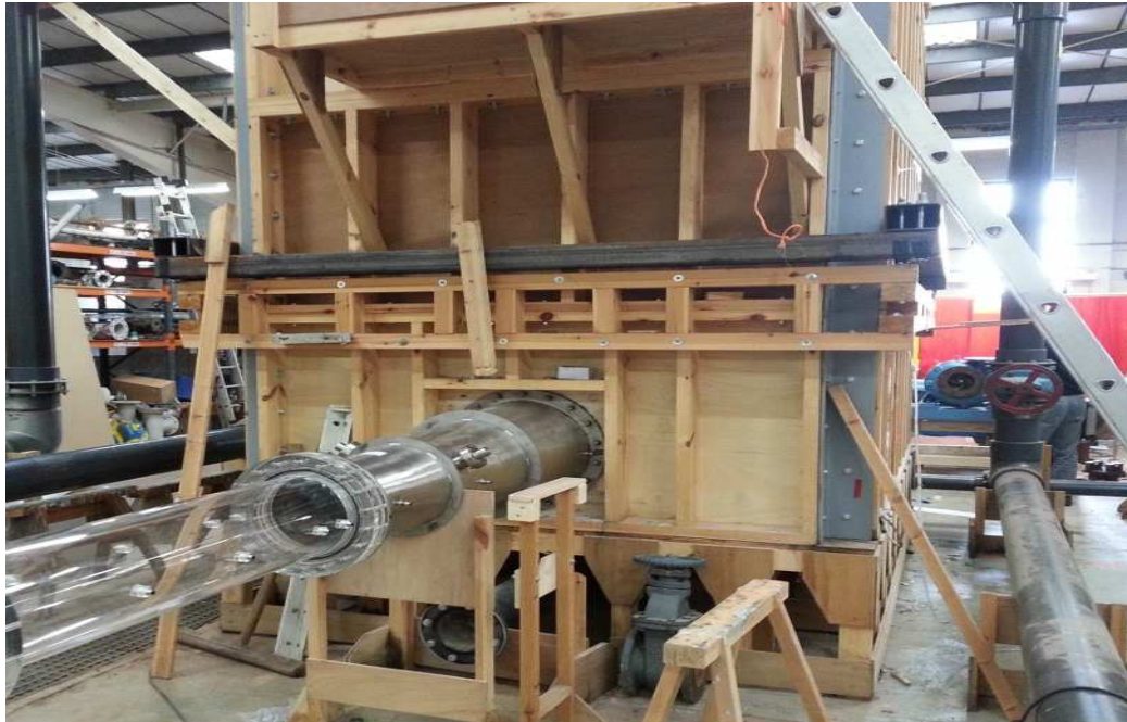
Figure 3: Header tank of experimental rig at BHR Group hydraulics laboratory
